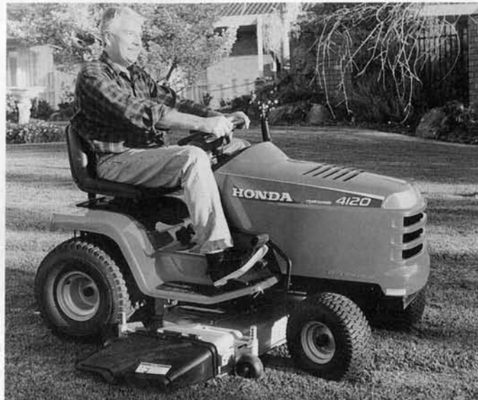
The commercial quality Honda HA4120 ride-on mower features a 122 cm width cut and is powered by the 14.9 kw(20hp) OHV GXV 620 engine.
